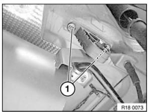
Release hexagon bolt (1) for supporting rear silencer/muffler at outside rear on left and right of body.
