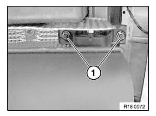
Release hexagon bolt (1) for supporting rear silencer/muffler at inside rear on left and right of body.
